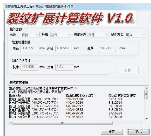
图 6 裂纹扩展计算结果 Fig.6 Computation of flaw growth.
